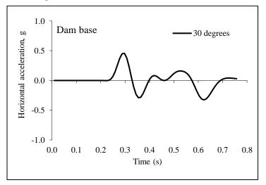
Figure 5. Response of base of dam to inclined SV wave for soil type D bounded by rock.
