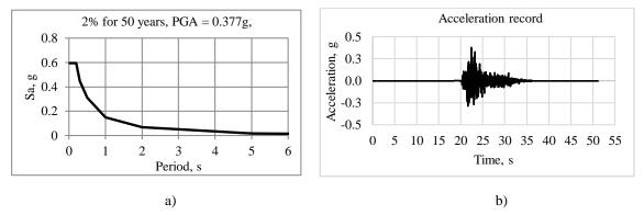
*Figure 3. a)* Acceleration spectrum for soil type C, b) Acceleration time history for soil type C.
