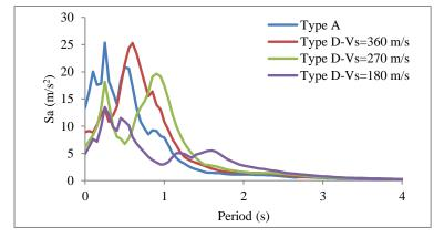
Figure 4. Spectral acceleration for different values of the shear wave velocity Vs.
